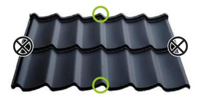
**Sheet Carrying.** The sheets should be carried by holding the ribs (green). Do not carry the sheet by the edges (black), as this may cause gaps in the side laps.
